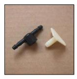
The LPI System uses a two component porting adapter comprised of a pedestal and a tee. The pedestal is secured to the surface over the void. Th barbed tee fits onto the pedestal to plumb the tubing.
