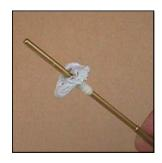
A special tool (M-260) is used to set the pedestals, It holds the pedestal as the epoxy is applied, and protects the opening into the void from oozing epoxy that may otherwise clog it. The M-260 Setting Tool also quides the pedestal to it's precise location.
