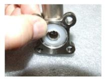
6. Install the exterior seal (S-332) with the spring groove facing away from the ball.
