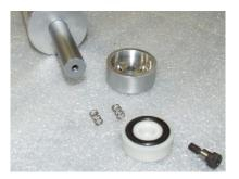
3. Remove the piston pad, springs, and piston pad holder from the metering piston. Be careful not to loose the springs. 4. Unscrew the metering piston retaining nut and remove.
