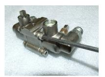
9. Attach the valve body to the spacer block. Take care not to distort the o ring seal. Snug, but do not tighten, the bolts until after the coupler shaft is installed. 10. Bolt the valve assembly back to the frame. Be sure that the ball valves are oriented properly.
