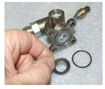
**Cleaning** Clean the components thoroughly, but do not use steel bristle brushes or instruments likely to scratch or gouge. Most solvents and cleaning agents can be used without damage to the stainless steel parts.
