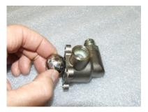
5. Slide the ball into the pocket with the detent (slot) facing the coupler pocket. Use the tang of the coupler shaft (M-581) to squarely align the ball slot.
