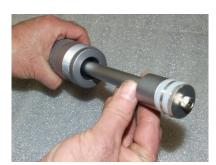
5. Now the piston can be removed from the metering cylinder. 6. To replace the piston seals, remove the screw in the cap retaining the seal. Then remove the cap, the seal, spacer, and the second seal.
