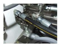
1. Using a 7/8" wrench,<br/>remove the inlet and<br/>outlet hose from their<br/>respective fittings at the<br/>COCO valve.2.
