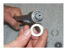
7. Seal spacer removed.
