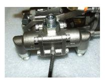
5. With a 3/16" Allen wrench, remove the bolt securing the spacer block to the frame module.
