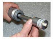
11. Slide the metering piston back into the metering cylinder, small end first.
