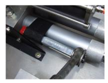
2. Loosen and remove the metering cylinder by rotating it counterclockwise. Do not use a pipe wrench! Use a strap wrench. 2. Remove the shoulder screww holding the piston pad in place. Be careful not to loose the springs located beneath the white plastic pad.
