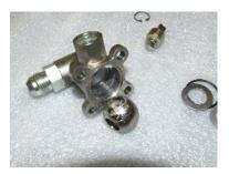
12. Now the ball can be removed from the housing. Inspect the ball looking for wear or scratches in the surface. Replace if needed. 13. Use the seal pick to remove the lower seal from it's seat. Take care not to scratch the seat.
