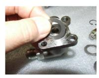
1. Fit the seal spring (S-330) into the pocket with its concave side toward the ball.12. Remove the lower 2. Place the washer (S-329) over the spring. Nudge it to be certain that both it and the spring are fully seated.
