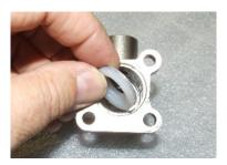
3. Insert the seal perpendicular to the bore until it is within the pocket. Then, twist it flat so that the spring side of the seal is facing down. 4. Nudge it into place with the fingers, and then press it firmly into the bottom of the pocket with the setting tool (M-806) from the seal kit.
