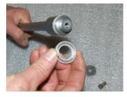
9. Be sure to install the seals with the metal springs facing out, towards the piston seal retainer. 10. Install the piston seal retainer and retaining nut.
