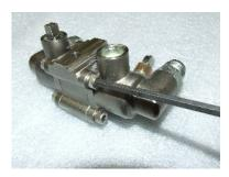
5. With a 3/16" Allen wrench, remove the four bolts that hold the ball valve body to the spacer block.
