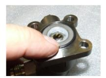
8. Press a new o-ring into the groove around the outside of the spring and washer. Use silicone lube to hold it in place.
