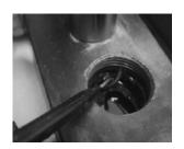
Apply an an anti-seize compound to the cylinder threads, and then screw it into the manifold. Do not overtighten!
