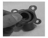
1. Fit the seal spring (S-330) into the pocket with its concave side toward the ball.
