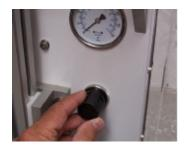
The pressure regulator at the front of the machine is adjusted by rotating to the right (clockwise) to increase the dispense pressure. Increasing the dispense pressure will incease the flow of material from the static mixer. Turning the regulator to the left (counter clockwise) decreases the dispense pressure. The knob locks into place when pushed in and must be pulled out to adjust the pressure.
