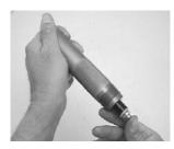
7. Lubricate the piston and chamber with silicone and insert the piston pad end first into the bottom (threaded end) of the metering cylinder.
