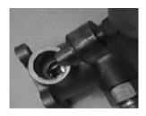
11. Carefully insert the coupler shaft (M-581), bronze bushing (M-802) and washer (P-469) into the housing.
