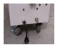
The electrical connection is located on the front (handle side) of the machine. The electricity is used to power the heater inside the cabinet. The electric heater requires less than 10 amps of 110v or 240v AC voltage.
